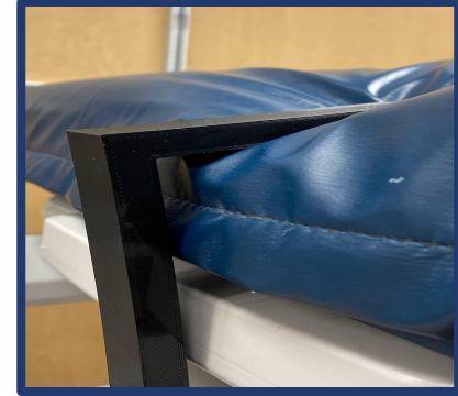
Bending and inadequate surface area on bed
