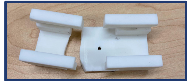
Lack of material allowed easy breaking
