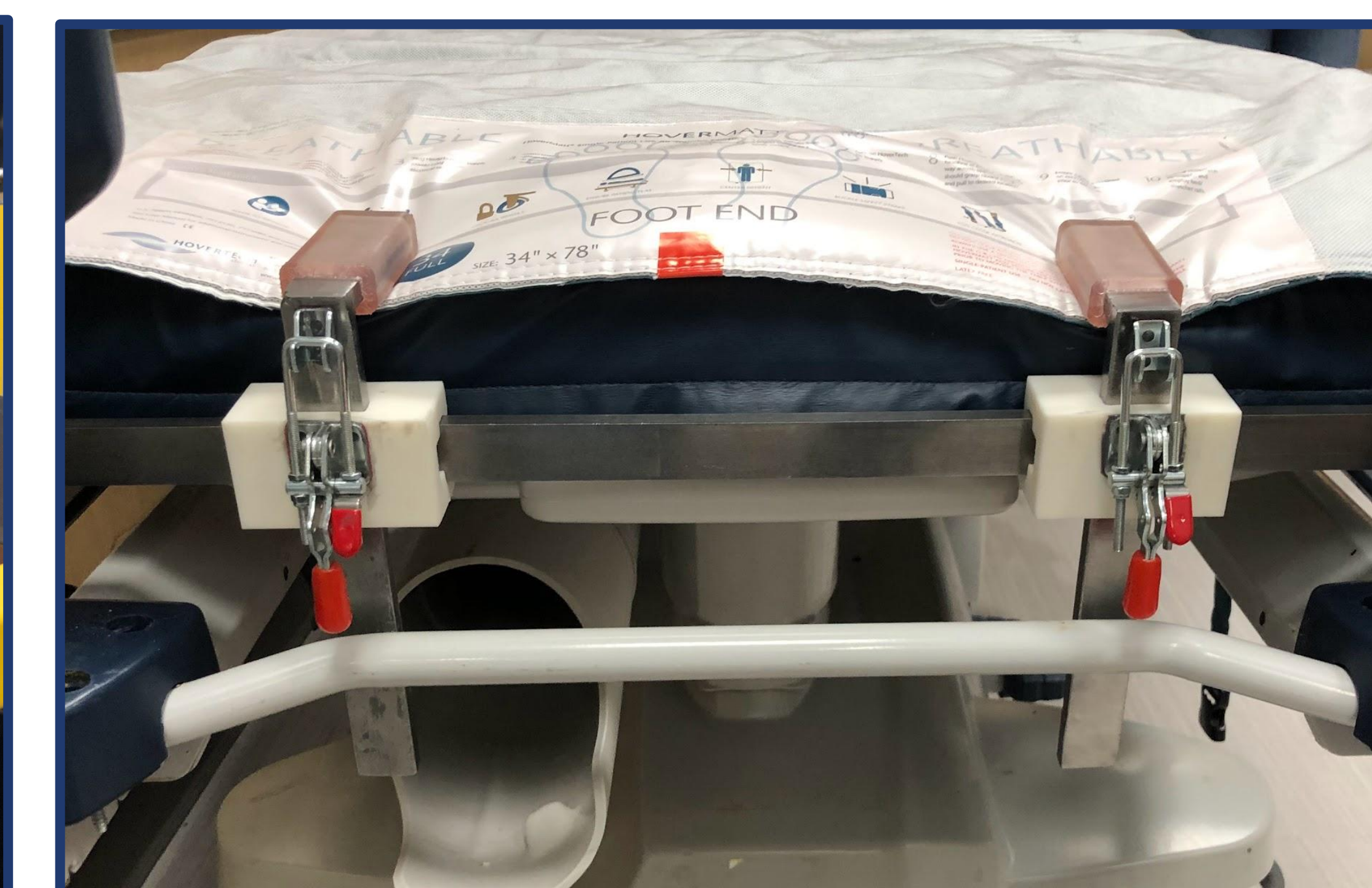
Figure 5. Testing setup for 2 clamps at the foot of a stretcher to hold the HoverMatt in place while the bed is tilted to 40 degrees with a test subject lying on top.
