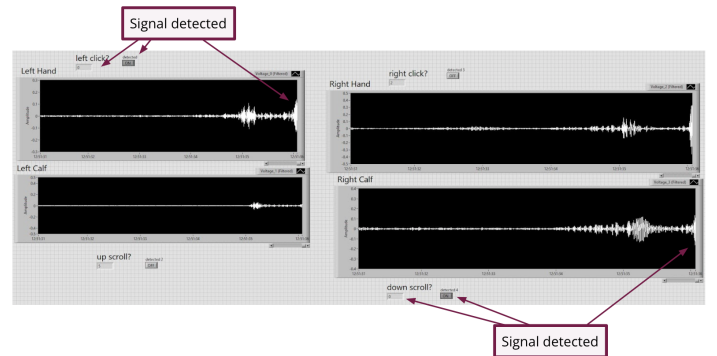
Fig. 6 – Screenshot of the front panel in LabVIEW. In this example, the right calf and left hand have EMG signals which surpass the Peak Detector VI's threshold value, resulting in a left click and down scroll command.
